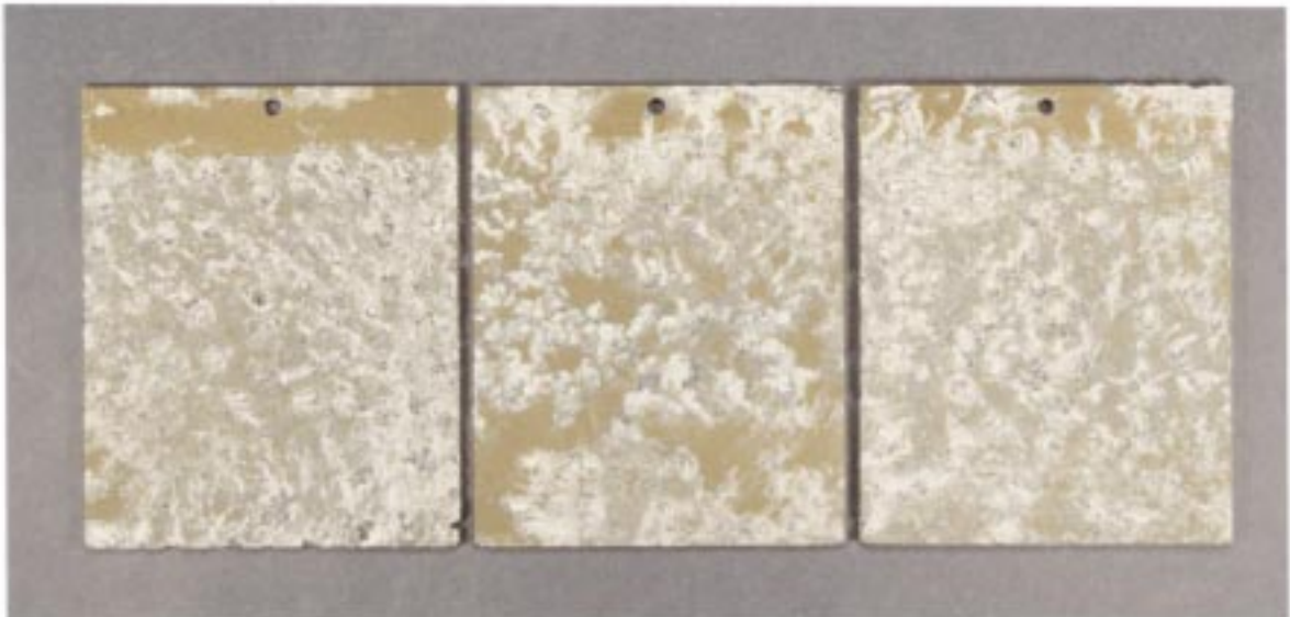
Figure 8 ZE41 Test Panels coated with type II coating and exposed to ASTM B117 salt spray test for 336 hours a) TAG 8200, b) HAE, c) Dow 17
