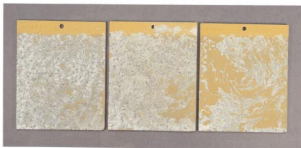
Figure 7 ZE41 Test Panels coated with type I coating and exposed to ASTM B117 salt spray test for 168 hours a) TAG 8200, b) HAE, c) Dow 17
